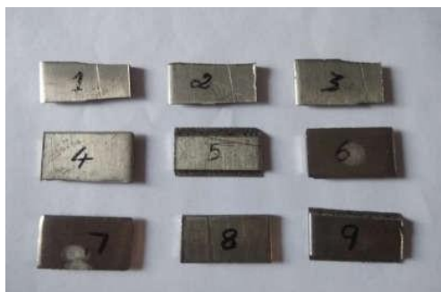
Fig 4: Monel 400 after Machining
