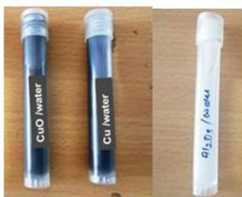
Fig.2 Prepared Nanofluids samples
